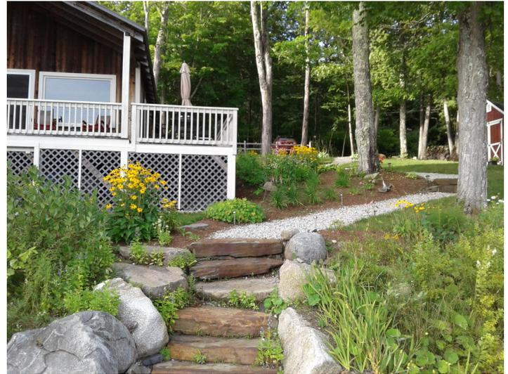
They allowed only a 5 – 6-foot opening for the stone stairs. Their driveway used to dive straight down to the shoreline and would wash sediment directly into the lake with every rain storm. The repair eliminated the driveway and a new curved stone pathway acts as a water bar to slow all runoff from reaching the lake. The results of all this work took their property from being a runoff disaster to becoming a poster child for Lake Wise.
